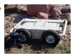
2. Turn Power OFF when not in use. Make sure you turn the power OFF at the MT-7X platform first, then the controller can be powered OFF.
