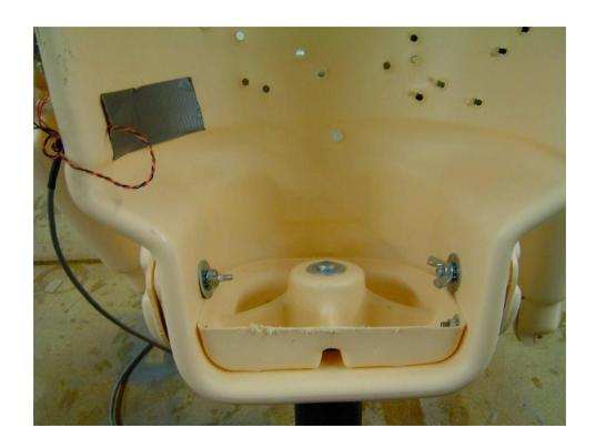
The bottom end of the pole is keyed to keep the mannequin aligned. The back of the pole has an indication line, this line marks key slot for the pole. This indicator marks the back of the pole. The bracket has 4 tabs, one of which is ½" taller than the rest, this is the key and is the rear of the unit. When installing the post into the mannequin, align the mark before tightening the screw.
