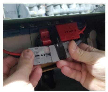
at 24V. The combination of batteries supplies 24V. The unit will operate down to 14V (7V in each pack) before under-voltage shutdown occurs. However, at this low voltage, the unit will move much slower and operation is not recommended due to the possibility of battery deep discharge.
