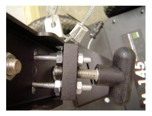
After loosening the hand knob, grab the knob and bar attaching the U-Bolt in the palm of your hand pressing the U-Bolt as far through the bracket as possible. Guide the 2 Pins into the matching holes in the post and the U-Bolt into the slot. You will feel the Latch engage. If the latch does not engage, loosen the hand Knob further and retry.
