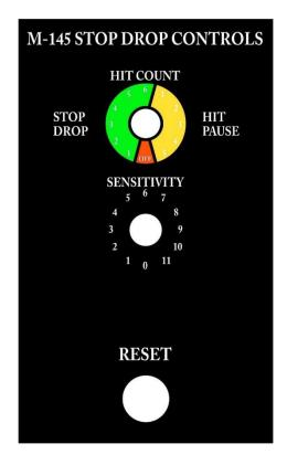
The top knob controls 3 modes. When set to 0 the post is disabled. Pressing the reset button with the knob set to 0 will cause the latch to disengage. Positions 1-6 control Hit-Stop/Drop mode with the number controlling the number impacts to activate the latch. Positions 7-11 on the switch control the Hit-pause mode with 1-5 hits to activate.
