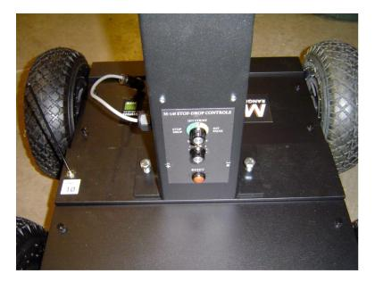
There are two Knobs on the post to control the hit settings. The top knob sets the count and mode. The bottom knob sets the sensitivity. Any time a change is to be made the power should be turned off. Upon power up, the reset button must be pressed to energize the post.
