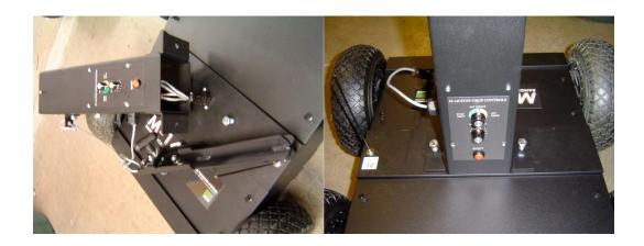
To remove a cover simply pull on each of the 4 plastic rivets until they click; about ¼" is all they move. The center Pin of the Rivet will stay in the fastener. When all 4 rivets are loose, grab 2 rivets on opposite sides of the cover and pull up.
