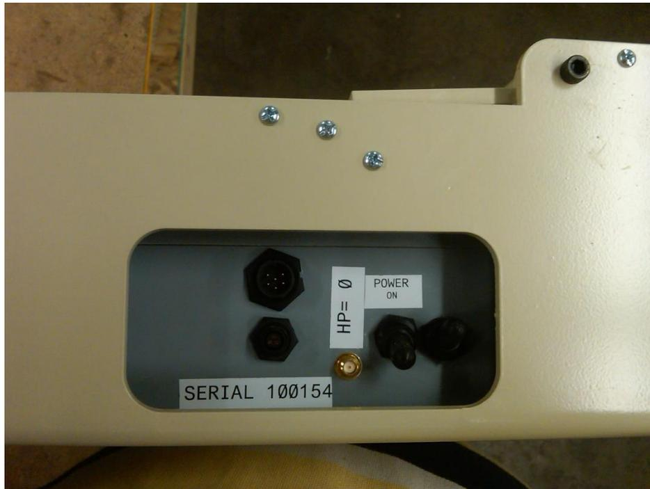
In the above picture the top port is the RS-485 Data and charging port. The bottom port is where the hit sensor plugs into.
