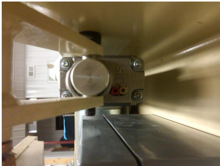
To adjust the retraction and extension you can turn the red and white screws on the end of the actuator. The Red screw adjusts the down position of the pushing arm. Turn the screw clockwise to make it arm retract further. The White screw adjusts the up position of the pushing arm, turn the screw counterclockwise to make the arm push further past 90 degrees. There are about +/- 10 turns of adjustment for each screw.
