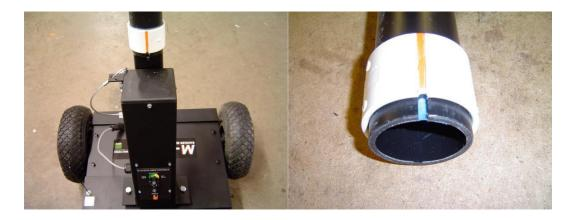
The M-145 is a Cost Effective Light Duty Robotic Platform designed to be quick and agile. The unit has a limited carrying capacity of 35#. A mannequin weights approximately 9 pounds. Overloading the M-145 will make it harder for the unit to turn and accelerate, decreasing performance. The more weight placed on the M-145 the shorter battery life will become.
