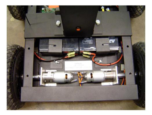
Caution: When charging you MUST remove both sets of battery cables from both batteries before connecting the charger; Failure to do so will cause damage to the charger, wiring and robotic platform.
