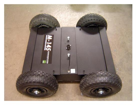
Note the location of the power switch on the side. The antenna is mounted on the top deck.
