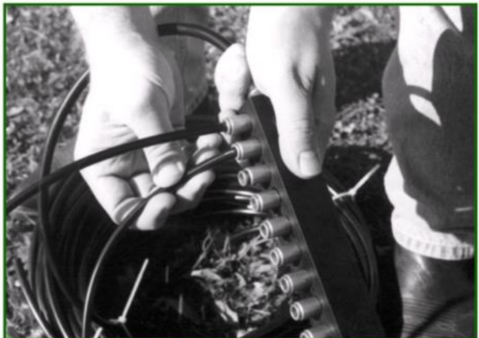
ILLUSTRATION 12: CONNECTING THE INDIVIDUAL TARGET AIR TUBES TO THE AIR MANIFOLD
